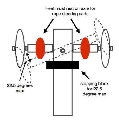
The above stopping block MUST be in place.
